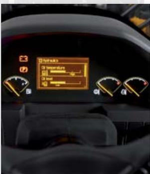
**Refined computer programming** will alert operators when regeneration needs to occur. Operation is possible while the machine regenerates, thus reducing downtime.
