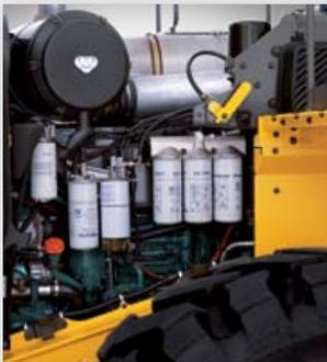
**Quality components and strategic placement of filters** provides for easy service, keeping machine downtime at a minimum and production time at a maximum.
